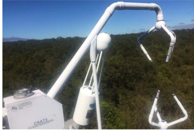
*A fluxnet micrometeorological monitoring station located in HAVO collects long-term environmental data.*
